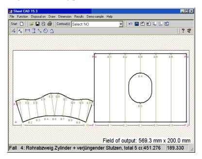
you can place the parts of unfolding further far away from the edge of sheet-metal plate. If you enter the desired distances and click the "**OK**"-button, then the parts of unfolding are moved:
