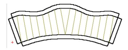
or seam edges of various widths will be appended to different sides of the sheet unfolding layout
