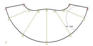
To measure an angle between two lines, mark first line, then a second line and afterwards the position of the dimension arc.
