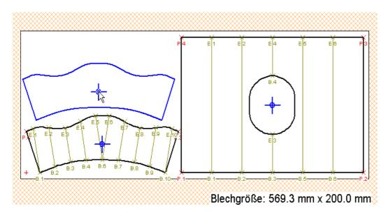
After the part is placed on the correct position, release the mouse button, then the part of unfolding is shown on the new place:
