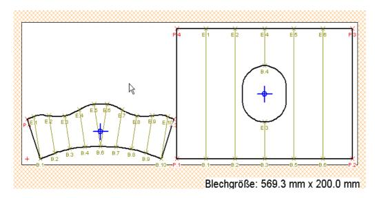
All parts have now a blue cross with circle. If you click with the mouse into the internal circle and keep the key pressed, then you can move this part within the sheet-metal plate at will.
