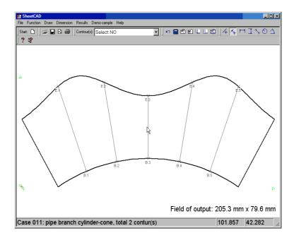
Select the required contour (see Section 5.1). Click on the option "**Optimize length of welded line**" in the menu option "**Edit**". The new sheet unfolding layout is displayed on the screen within a few seconds:
