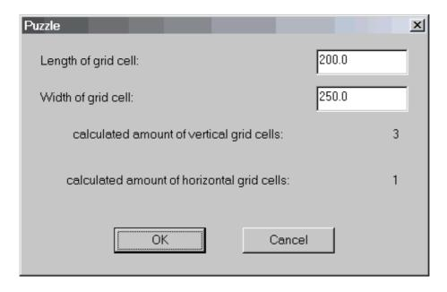
Enter the length in the window "length of grid cells" and the width in the window "width of grid cells" and the program will calculate automatically the number of fields required for the sheet unfolding layout. Confirm with "OK". The puzzle is displayed on
