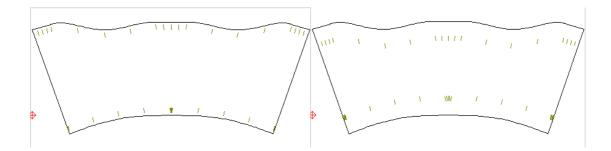
Enter the segment length. See the example of the sheet unfolding layouts with segment length = 2 mm and 13 mm:
