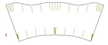
The sheet unfolding layout is displayed showing "the distance between the edge of segment" = 2 mm and 10 mm, for example.
