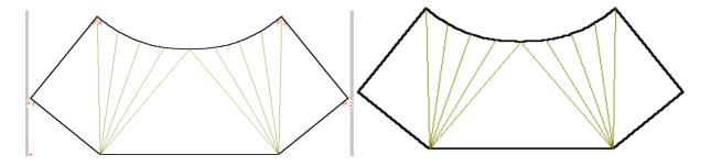
Enter here also the distance between the dashes and the length of the dashes for the sheet unfolding layout, using the dashes.
