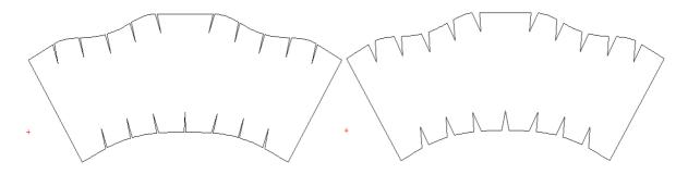
See example: Sheet unfolding layouts with "notch length" = 2 mm and 5 mm:
