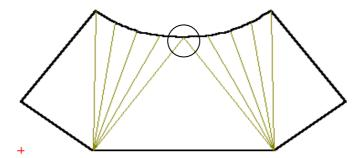
If command" **empty drawing for start and end fold lines**" is active, fold lines will be shown as follows:
