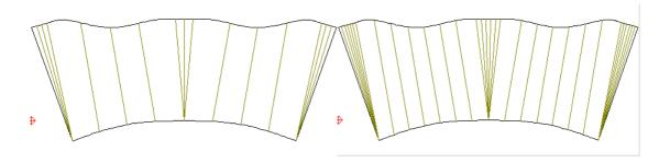
See example: Sheet folding layouts with ",Angle step" = 35 und 80 To change the number of fold lines, enter the required number and click on "OK".
