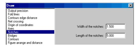
Enter the width and length of the notches and click "OK"-Button. The fold lines of the corresponding contour will be displayed using notches.
