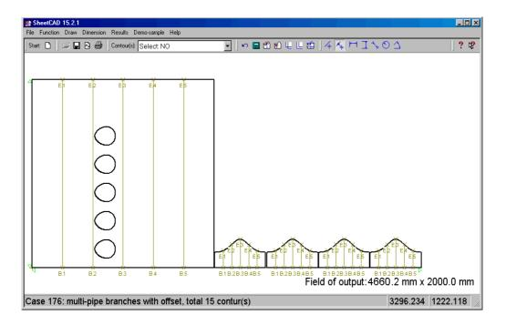
As "Distance to the edge of plate - left/bottom" and "Distance to the edge of plate - right/upper" enter here the distances between the edges to the outermost left and lower points (or outermost right and upper points of the contour) and the edges of sheet-metal plate in mm. Control mark  $\checkmark$  shows, which case is active.
