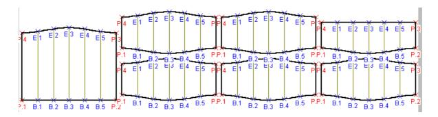
Under "Least distance between figures" enter the distance between sheet unfolding layouts in mm.
