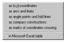
Click the corresponding option to view the sheet unfolding layout in one of these formats. The Windows Write Editor is loaded automatically and the corresponding text file is displayed on the screen: The following coordinate data will be shown:
