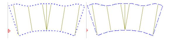
See example: Sheet unfolding layouts with bridge distance = 5 mm and 15 mm:
