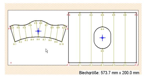
In order to rotate a part, place the cursor beside the cross-hair in the center of the desired part. Press the left mouse button; the contours are represented as strokes. Keep the left mouse button pressed and rotate you with the mouse the blue image of the part up to the desired position:
