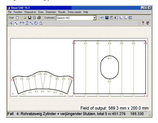
you can place the parts of unfolding further far away from the edge of sheet-metal plate. If you enter the desired distances and click the " $\mathbf{OK}$ "-button, then the parts of unfolding are moved:
