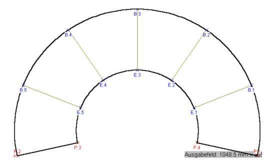
You can cut this unfolding across the bending lines and get 6 parts. Select the outside contour (see "Select contour"), the contour will be blue, and click the command "Regular divide" under "Edit", you get 6 parts on the screen:
