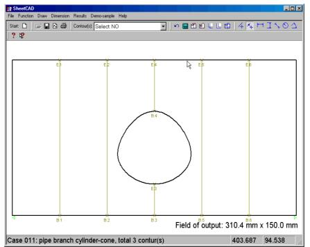
Select the desired contour (See Section 5.1). Click the option "Select position of welded seam" in the menu option "Edit". A blue line is displayed at the cursor. This is the welding line. Position the welding line using the cursor:
