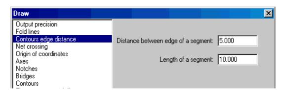
The ends of the fold lines are displayed as short segments with their distance from the contours. Enter the border distance and the length of the segments in the mask of the sheet unfolding layout.
