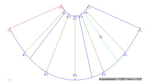
When all lines are placed on the required places, you can start the cutting by clicking the right mouse-button. The unfolding will be cut automatically:
