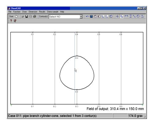
**Note:** The welding line angle of between  $0^{\circ}$  and  $360^{\circ}$  is displayed in the bottom left-hand corner of the screen to enable correct positioning.
